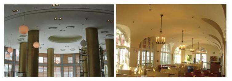
Sonacoustic<sup>®</sup> conforms to any surface: Flat, Vaulted, Domes and Curves.
